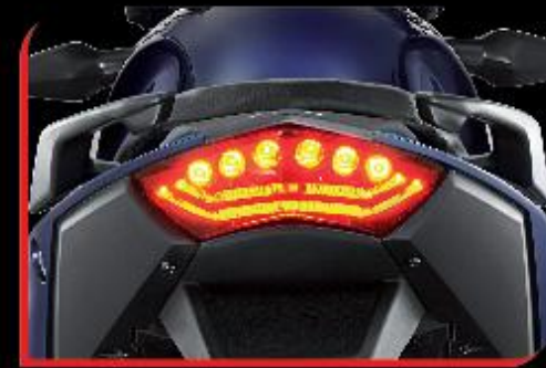
NEW TAIL LAMPS WITH LED LIGHT GUIDES
